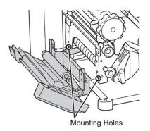
7. Fasten the two Fixing Bolts and two Screws to secure the Label Peeler Module, and then close the module's Front Cover (fastened by 0.74 Nrm ± 0.10 Nrm).
