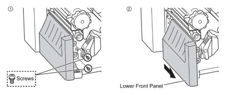
3. Remove the two Screws and then remove the Lower Bar.
