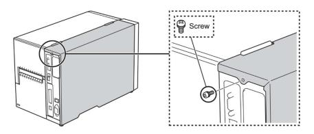
2. Remove the PCB Cover by pushing it toward the back of the printer, and then lifting it with both hands.
