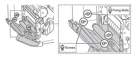
8. Fasten the remaining two Screws on the module's Front Cover as illustrated (fastened by 0.74 N • m ± 0.10 N • m).
