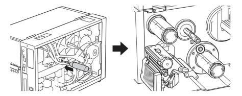
4. Install the Media Guide Bar and Rear Label Guide Module and use a 13 mm spanner or a 1/2 inch wrench to fasten it.
