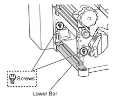
4. Remove the Black Cap. Install the Roller Module in the slot, and fix the Screw as illustrated (fastened by 0.74 N • m ± 0.10 N • m), and then insert the Black Cap back into the slot.
